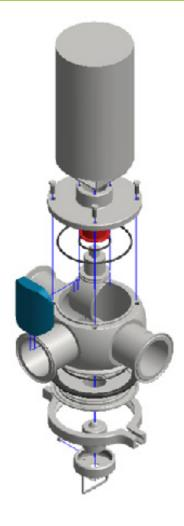
LIAG<sup>®</sup> EASY-OPEN arc valves are specially designed as reliable component of inline metal detectors and process lines in the meat industry without CIP Cleaning. This valve performs easy and quick opening with excellent cleanability.
